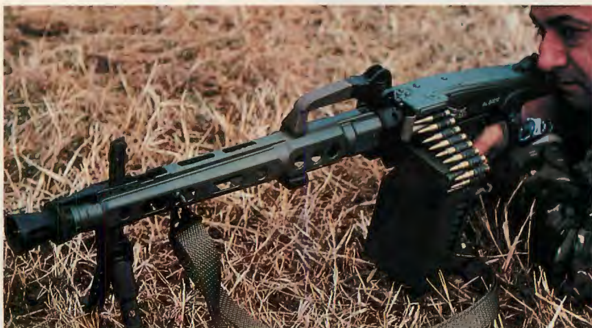
TOP: CETME MG82 in assault-carry position. LEFT: Spanish soldier moves forward during field trials with MG82. ABOVE: CETME MG82 has cyclic rate of fire of 900 or 1,250 rpm. RIGHT: MG82 shows outward characteristics of MG42, weighs 14.8 lbs. empty and is 36.6 inches long.
